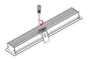
Tighten the screws. Installing other buckles in the same way
